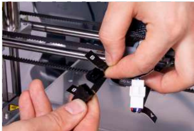
Connect the extruder 'A' cable to the 'A' plug and the 'B' cable to the 'B' plug on the X carriage.
